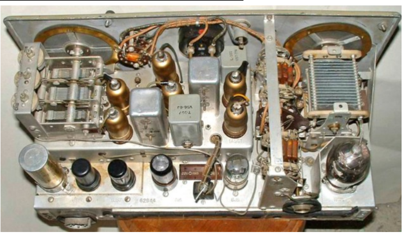
Top view of V-100-B chassis. Note that the receiver section is a separate assembly. The original USA receiver valves were probably at a later stage replaced by valves from Soviet production.
